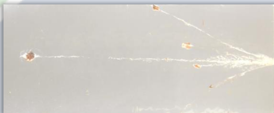
.40 S&W PISTOL CARTRIDGE 10% BALLISTIC GELATIN
