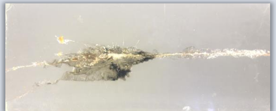
300ACC BLACKOUT RIFLE CARTRIDGE 10% BALLISTIC GELATIN
